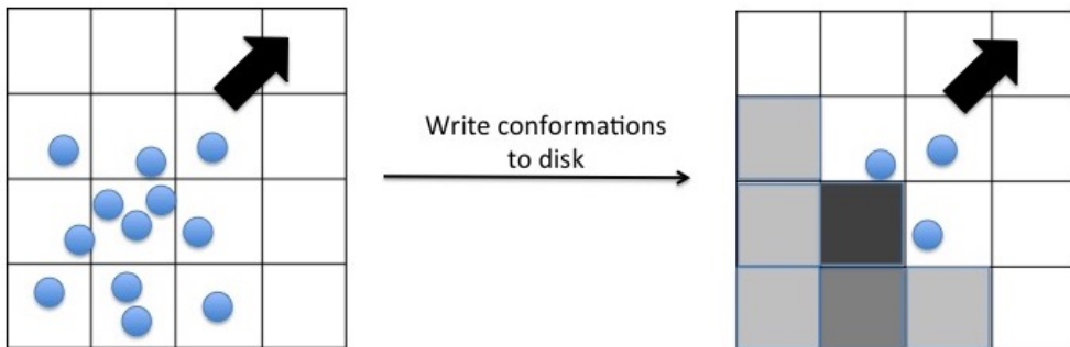
Figure 1: Pictorial representation of the effect that the use of summarized coverage statistics has on a local coverage grid. Each blue dot represents a previously sampled conformation. Before hitting memory limits, the exploration is proceeding in some direction depicted by the black arrow. When the exploration restarts, summary coverage statistics are maintained and depicted in shades of gray. Darker shades indicate more densely sampled areas that the algorithm can use to reduce sampling redundancy.
