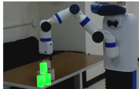
Fig. 8: The Fetch received a HARS to stack three wooden cylinders on a table. The arrange of virtual cylinders can be observed superimposed the real cylinders.
