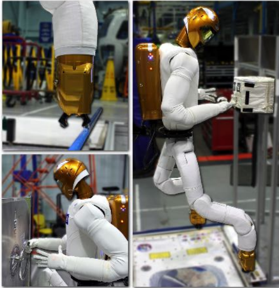
Figure 1. NASA's Robonaut 2 executing geometric constrained manipulation tasks. Clockwise from the top-left: R2's end-effector moves on the Z-axis to grasp a handrail, R2's legs form a closed-chain and a cargo bag is moved linearly from its hold, and R2 turns a valve about its axis.
